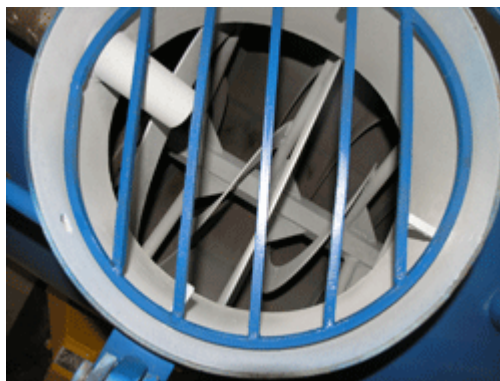
View of internal part of the mixer through the loading nose section.
